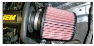
18. Install the AEM<sup>®</sup> air filter onto the intake tube and secure with the provided hose clamp.
