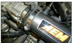
16. Install the AEM<sup>®</sup> intake tube into the heat shield and then into the coupler, adjust the tube for best fit and secure with the provided hardware.
