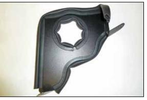
12. Install the edge trim onto the heat shield as shown.
