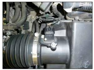
4. Disconnect the mass air sensor electrical connection.
