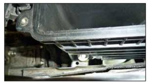
9. Loosen the bolts that secure the lower air filter housing and then remove the lower housing from the vehicle.
