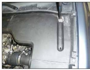
2. Remove the pins that secure the drivers side rear decorative engine cover and then remove the cover.
