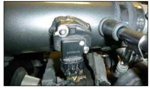
17. Reconnect the mass air sensor electrical connection.
