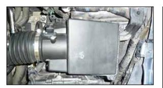
7. Loosen the four bolts that secure the upper air filter housing and then remove the upper housing and intake boot.
