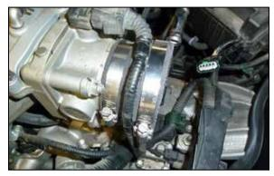
15. Install the provided coupler (084034) onto the throttle body and secure with the provided hose clamps.
