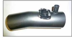
10. Remove the mass air sensor from factory air filter housing and then install into the AEM<sup>®</sup> intake tube and secure with the provided hardware. Install the crank case vent adapter grommet into the AEM<sup>®</sup> intake tube as shown.
