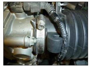
6. Loosen the hose clamp that secures the factory intake boot to the throttle body.
