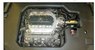
19. Reinstall the decorative engine covers and reconnect the negative battery cable.
