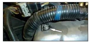
13. Remove the wiring harness mounting bolt shown on the shock tower.
