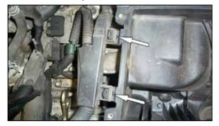
8. Unclip the wiring harness from the lower air filter housing.
