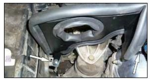
14. Install the heat assembly and secure with the provided hardware.
